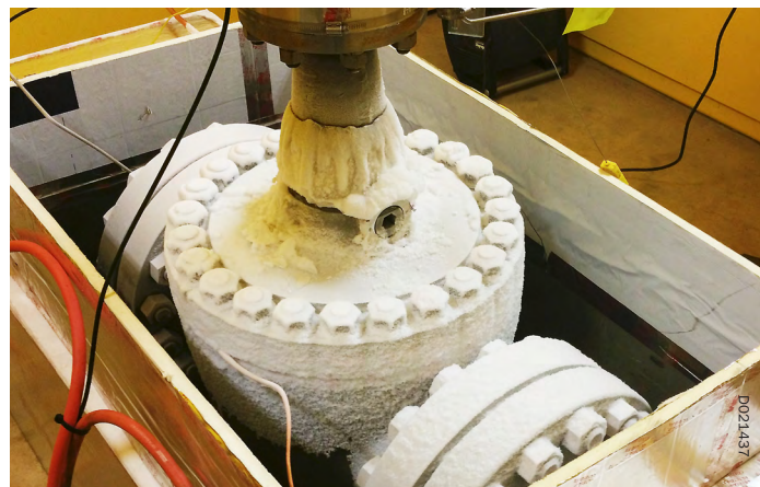
Testing is performed on a variety of products to determine operation and seal integrity at temperatures as low as -320°F.
